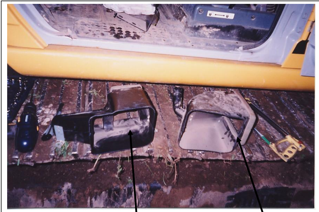
Retain and reinstall after the heat/cool box has been mounted. Seal to the box with tar tape and self adhesive foam tape. Cut with a knife or hack saw. The retained section is approximately 8 6" long
