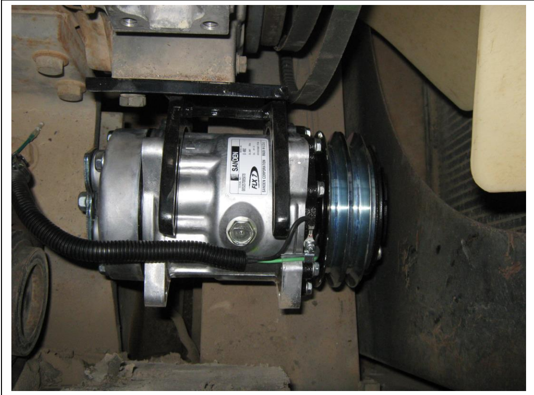
Compressor placed on mount.
