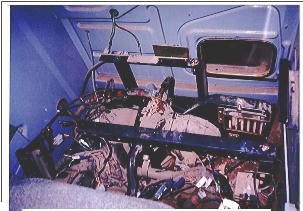
Heater still in place with all the necessary parts removed from above it.
